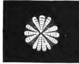
FIG. 5 (after Dippel). Transverse section of a tracheide of Pinus sylvestris viewed with crossed Nicols.
